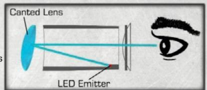
Opposed to a normal riflescope, a canted objective lens is integral to the function of reflex optical sights. The LED is positioned near the base of the housing, close to the first lens. The objective lens is canted towards this emitter to properly reflect the light given off from the LED back to the shooter and create the dot image seen by the user.
