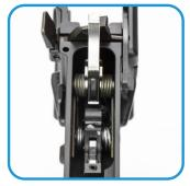
4. Install hammer, verifying spring legs are on top of the trigger pin. Cock hammer back.
