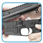
1. Verify firearm is unloaded and remove upper from lower receiver.
