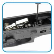
5. If hammer is captured by rear disconnector, adjust rear screw clockwise until hammer pops upward (audible click will be heard). Advance screw counter-clockwise 1/8 additional turn.
