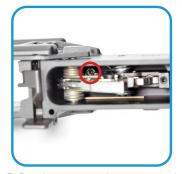
6. Once hammer is no longer captured by rear disconnector, depress trigger and hold. If hammer does not fall, loosen overtravel screw until trigger falls. Loosen additional 1/8 turn.
