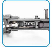
\*7. Adjust overtravel screw counter-clockwise until trigger fires. Once fired, additional turns will increase overtravel to your liking.
